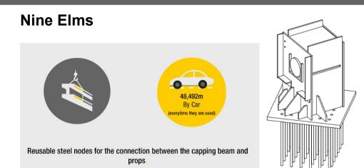
We have created a reusable steel nodes (shear blocks) for the connection between the capping beam and the reusable prop. Whilst these might appear CO2e intensive, by the end of the their second use they reach their carbon payback, and therefore become a truly sustainable solution. In future these nodes will save 15tCO2e every time they are used.
