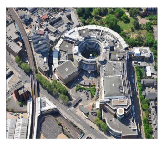
The McGee's scope of works included soft strip, asbestos, demolition of the central wedge area, Studios 4, 5, 6 and 7, the restaurant block, the drama block, including two 40 meter chimney stacks and the careful deconstruction of three Link bridge structures. On completion of the Studio structures McGee were awarded a ground works package which included installing a 150 meter perimeter sheet pile wall and perimeter ring road hard standing road.
